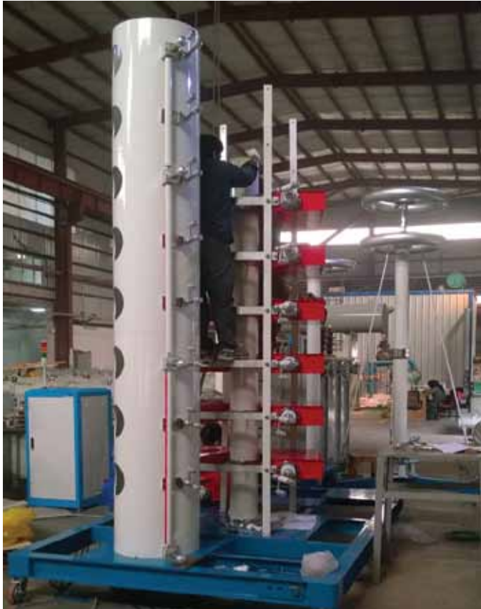
Impulse testing upto 800kV
